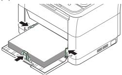
**Note** Load an amount of paper that fits under (does not contact) the tabs on the width guides.
